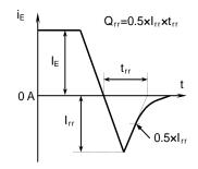
trr, Qrr characteristics test circuit and waveform
