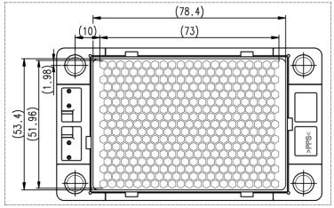
Dimension in mm, tolerance: ±1 mm
