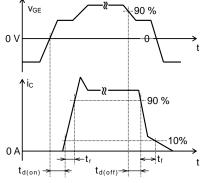
Switching characteristics test circuit and waveforms
